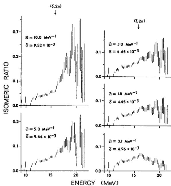
Fig. 1. The isomeric ratio for the reaction  $^{108}\text{Pd}(\gamma, n)^{107}\text{Pd}$ ,  $^{107m}\text{Pd}$ , obtained for five values of the level density parameter,  $a$ , used to correct the  $^{108}\text{Pd}$  photoneutron cross section for neutron multiplicity. The r.m.s. first difference,  $\delta$ , over the energy range 15.35 MeV to 17.10 MeV is given in each case. The  $(\gamma, 2n)$  threshold is indicated.
