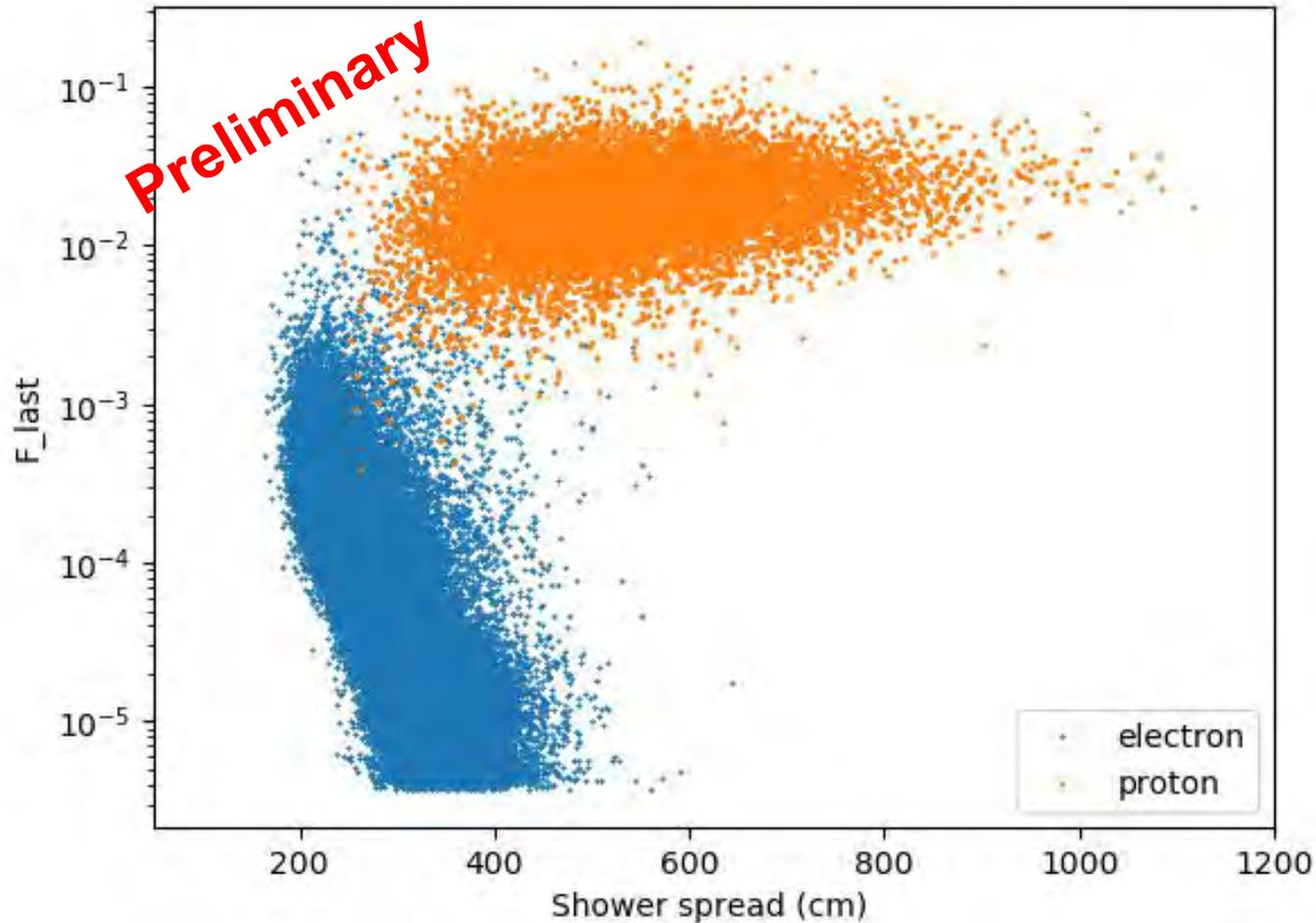
Proton rejection by  $> 99.99\%$  (for 90% electron eff.) at 500 GeV
