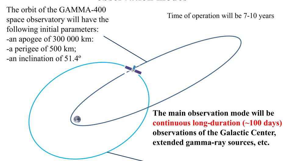
Under the action of gravitational disturbances of the Sun, Moon, and the Earth after ~6 months the orbit will transform to about circular with a radius of ~200 000 km and will be without the Earth's occultation and out of radiation belts.
