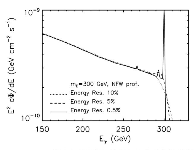
Energy resolution for Fermi-LAT is ~10% ( $E_{\gamma}$  > 10 GeV) and ground-based gamma-ray telescopes is ~15% ( $E_{\gamma}$  ~ 100 GeV)
